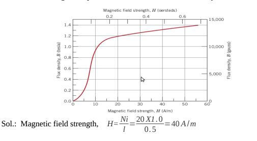
Magnetic flux density in vacuum,  $B_0 = \mu_0 H = 4 \pi X 10^{-7} X 40 = 502.4 X 10^{-7} T$
